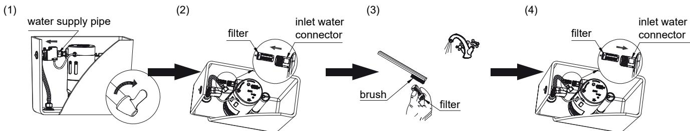
Shut off the water supply valve, then remove the water supply pipe.
